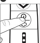
When done, push the Steam Level Power Button to the standby mode.
